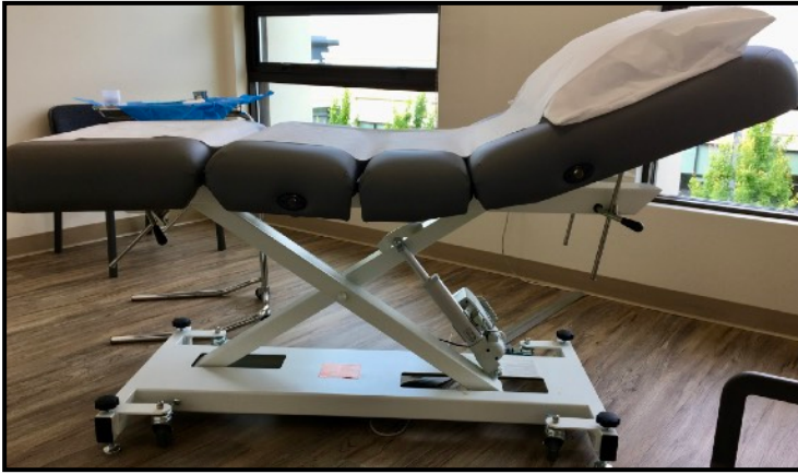
The bed at a doctor's office uses a hydraulic scissor lift!
